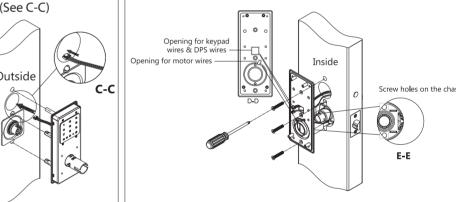
Step 9: Plug in the wires (keypad, DPS and motor wires) on the inside assembly. (See F-F)
