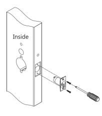
2 screws. (Optional) Install the Door Position Switch DPS into the frame.
