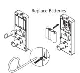
Press the pin wrench into the "RESET" hole on the inside subrose
