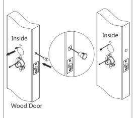
Step 6: (Optional) Install Interior Weather Gasket. Ensure all bumps on the gasket depressed into the round holes on the inside mounting plate. (Optional) Install Exterior Weather.
