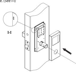
**Step 15:** Use a screw driver to rotate the cam in the post on the outside assembly until the cam is located
