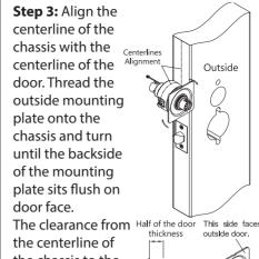
the chassis to the mounting plate is half the door thickness. (See A-A)
