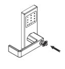
**Step 16:** Cylinder and outside lever installation. Insert cylinder into the lever first, and then insert the cylinder piece into the notch in the lever.
