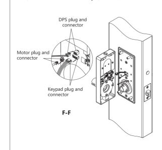
**Step 10:** Install the inside assembly with 4 screws. Be careful to not pinch wires. Once inside trim is secured, rotate the post to make sure there is no binding. Post should easily rotate back and forth, if jammed please check alignment from steps 3 & 4.
