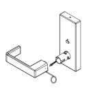
**3**: Rotate the lever in the opposite direction to change the handing.
