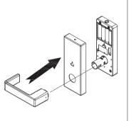
**Step 14:** Install the outside escutcheon plate first and make sure it snaps into place via the bumps on the sub rose. (See I-I)
