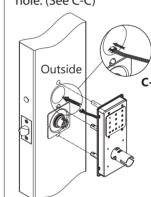
**Step 8:** Install the inside mounting plate. Route the wires (Keypad, DPS & motor wires) through cutouts indicated on mounting plate. (See D-D) Make sure the two bolts on the inside mounting plate pass through the vertically positioned screw holes on the chassis. (See E-E) Secure the inside mounting plate wit screws provided.
