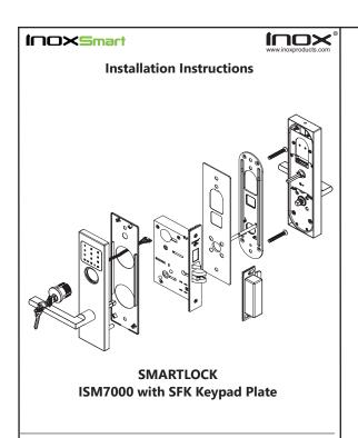
diagram, mechanical assembly drawings provided with each product, the local authority having jurisdiction (AHJ) and the National Electric Code, NFPA 70. When installed in fail secure mode, the local authority shall be consulted with regard to the use of possible panic hardware to allow emergency exit from the secure area.
