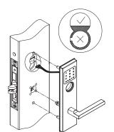
Mount the cylinder into the mortise lock. Do not tighten cylinder
