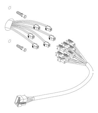
Install anchors. Pull molex wires through the center hole and connect according to wiring diagram. Keep any unused wires isolated and protected.
