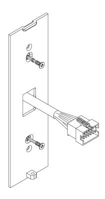
Install screws to mount the sub-plate.
