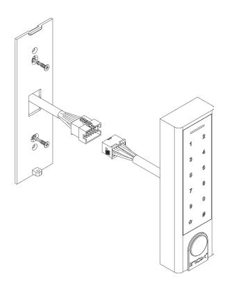
Connect the molex from the ISK-B300 with the molex from the locking device.
