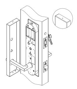
Slide the interior cover plate over the lever, push it onto the inside sub-plate and click the interior cover plate into place. Ensure the cover plate is securely attached by the ball bearing on top of the escutcheon
