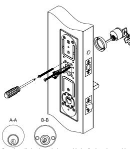
Pass the cylinder through the provided collar into the outside escutcheon. Make sure that the cylinder is orientated so that the mounting holes are positioned low as shown. Screws to secure the cylinder in place will pass through the interior subplate to tighten into position. Once the cylinder is secured, test the alignment by using the key to throw and retract the tubular deadbolt.
