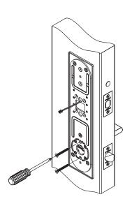
Partially screw in the top and bottom thru-bolt to the outside escutcheon plate. Throw the deadbolt to ensure that the deadbolt can be smoothly retracted.
