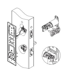
OPTIONAL: If installing the DPS, insert the DPS wire through its designated hole and pull it through the inside trim above the latch.
