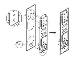
Additionally, make sure the bumps at the top and bottom of the gasket align and fit into the corresponding small round holes on the installation plate.
