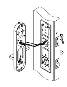
Firmly plug the wire into the socket of the inside plate. There is an audible "click" when the wire is properly inserted.
