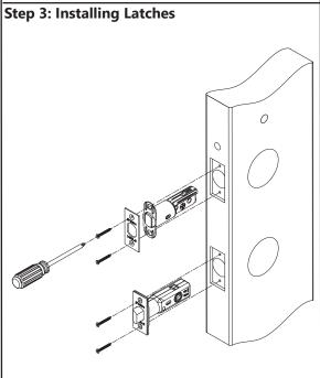
Attach the two faceplates with the provided screw packs using a Phillips screwdriver.
