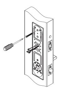
Tighten the M6x30mm machine screws from the inside installation plate.
