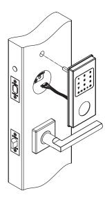
Depending on the CTC (Center-to-Center) placement, the wire should be routed as follows:
