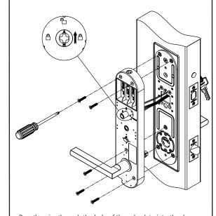
Pass the wire through the hole of the sub-plate into the door before mounting the inside plate.
