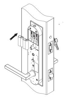
Ensure that the deadbolt is in the retracted position before installing the four (4) AA batteries. Align the batteries to the correct polarity in the compartment.
