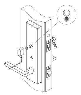
Place the clear washer onto the thumbturn hub. Align the thumbturn set screw to the groove of the spindle. Tighten the set screw using the Allen key.
