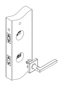
Insert the interlocking bracket into the bottom hole and the lever spindle into the tubular latch.
